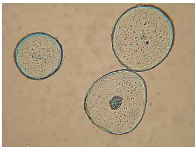
Figure 5 Photomicrograph of the white human hair treated with 5.0 wt % hydrolyzed protein derived from fish collagen (HCP) at 50°C for 1 h, then cross-sectioned, and finally dyed with methylene blue. [Color figure can be viewed in the online issue, which is available at wileyonlinelibrary.com .]
