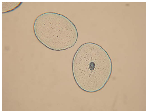
Figure 3 Photomicrograph of the white human hair treated with 1.0 wt % Glycine (Gly) at 50°C and pH 7.0 for 1 h, then cross-sectioned, and finally dyed with methylene blue. [Color figure can be viewed in the online issue, which is available at wileyonlinelibrary.com .]
