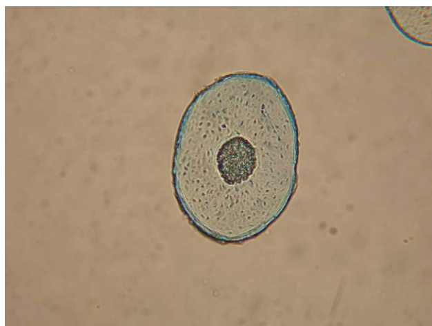
Figure 4 Photomicrograph of the white human hair treated with 5.0 wt % hydrolyzed protein derived from eggwhite (HEWP) at 50°C for 1 h, then cross-sectioned, and finally dyed with methylene blue. [Color figure can be viewed in the online issue, which is available at wileyonlinelibrary.com .]
